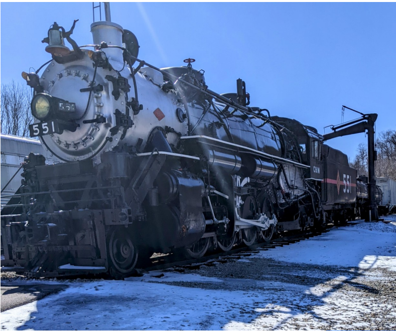
Left and below: The 1928 Chicago & Illinois Midland Railroad Steam Locomotive #551 was a 2-8-2 Mikado built by Lima Locomotive Works. Big and powerful, its name was changed from Mikado to McArthur during WWII. This engine powered coal trains from Illinois Midland Coal Mines to Commonwealth Edison Electric Generating Plants.
